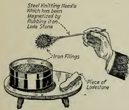
FIG. 24.—Piece of steel darning needle (which has been magnetized) attracting iron filings.
